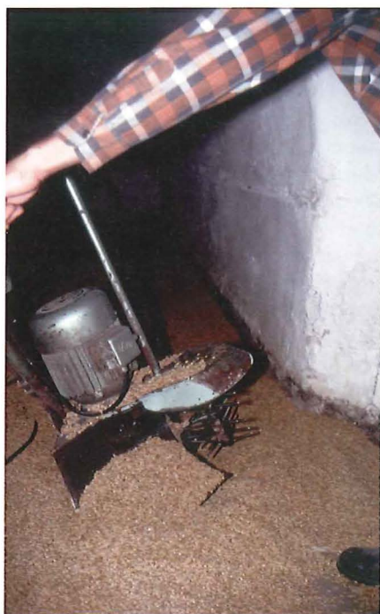
A hand-guided machine turns the malt over as it dries.
