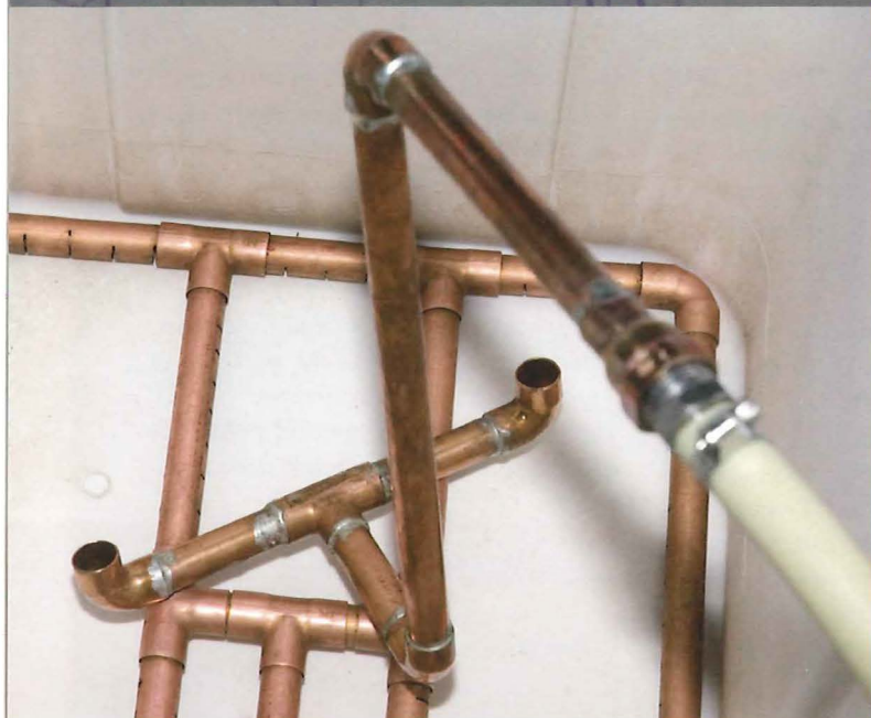
Copper recirculating arm leading back to the Igloo Cooler lauter tun
